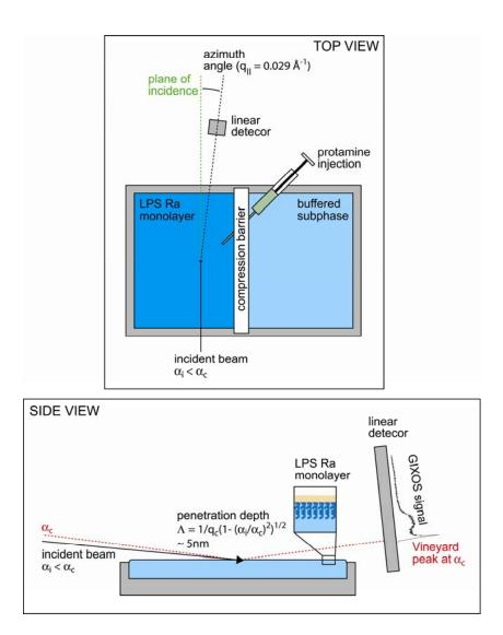
Schematic illustrations of the GIXOS setup: top view (upper panel) and side view (lower panel).
