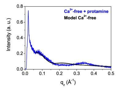
GIXOS curve and the reconstructed electron density profile of the LPS Ra monolayer on  $Ca^{2+}$ -free buffer after the protamine injection (blue). The measured curve can not be represented by any slab model. Such as the best-fit model of the same monolayer without protamine (black), indicating that the layered structures of the film were completely disrupted.
