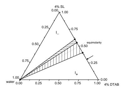
**Figure S2.** Schematic ternary phase diagram of the SL / DTAB system at 25°C (the arrow represents our starting solution (reference sample; mass ratio 30 / 70).
