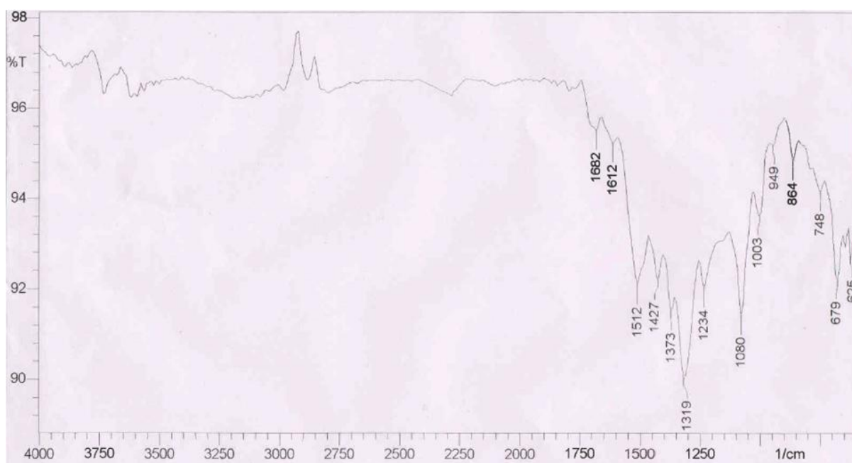
Figure: S1(c) IR Spectrum of [\text{Cr} (\text{C}_{36}\text{H}_{36}\text{N}_4) (\text{OAc})] (\text{OAc})_2
