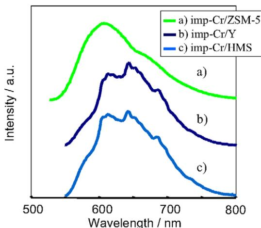
Fig. 3. The photoluminescence spectra of (a) imp-Cr/ZSM-5 (Si/Cr = 100, SiO<sub>2</sub>/Al<sub>2</sub>O<sub>3</sub> = 1880), (b) imp-Cr/Y (Si/Cr = 100, SiO<sub>2</sub>/Al<sub>2</sub>O<sub>3</sub> = 260), and (c) imp-Cr/HMS (Si/Cr = 100).
