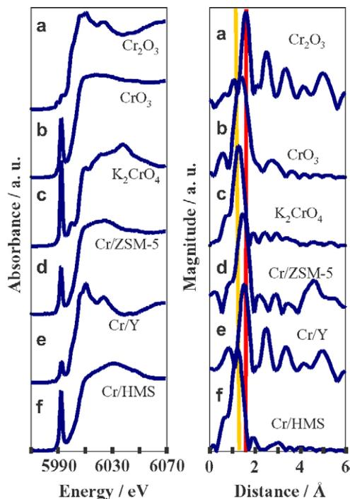
Fig. 1. XANES (A–F) and FT-EXAFS (a–f) spectra of (a)  $\text{Cr}_2\text{O}_3$ , (b)  $\text{CrO}_3$ , (c)  $\text{K}_2\text{CrO}_4$ , (d) imp-Cr/ZSM-5 ( $\text{Si}/\text{Cr} = 100$ ,  $\text{SiO}_2/\text{Al}_2\text{O}_3 = 1880$ ), (e) imp-Cr/Y ( $\text{Si}/\text{Cr} = 100$ ,  $\text{SiO}_2/\text{Al}_2\text{O}_3 = 260$ ), and (f) imp-Cr/HMS ( $\text{Si}/\text{Cr} = 100$ ).
