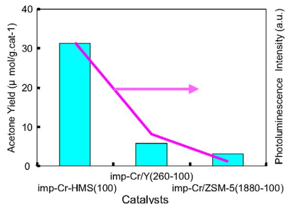
Fig. 4. The intensity of photoluminescence and the yields of acetone in the photocatalytic oxidation of propane with O<sub>2</sub> on imp-Cr/ZSM-5 (Si/Cr = 100, SiO<sub>2</sub>/Al<sub>2</sub>O<sub>3</sub> = 1880), imp-Cr/Y (Si/Cr = 100, SiO<sub>2</sub>/Al<sub>2</sub>O<sub>3</sub> = 260), and imp-Cr/HMS (Si/Cr = 100) under visible light irradiation ( $\lambda > 450$  nm).
