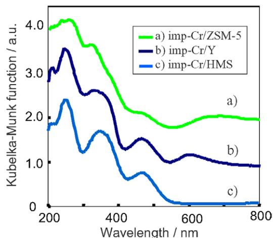
Fig. 2. Diffuse reflectance UV–VIS spectra of (a) imp-Cr/ZSM-5 ( $\text{Si}/\text{Cr} = 100$ ,  $\text{SiO}_2/\text{Al}_2\text{O}_3 = 1880$ ), (b) imp-Cr/Y ( $\text{Si}/\text{Cr} = 100$ ,  $\text{SiO}_2/\text{Al}_2\text{O}_3 = 260$ ), and (c) imp-Cr/HMS.
