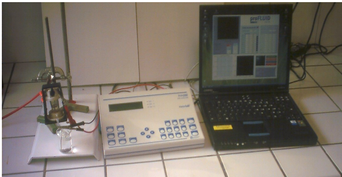
Fig. 3. Photography of the new semi-automatic SP measurement apparatus and its software proFluid 1.2 (university of Angers, UMR-MA105, Feb. 2006).
