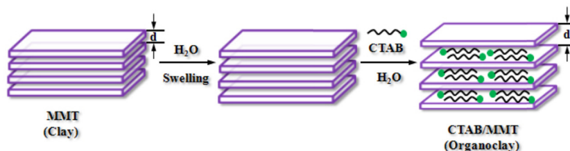
Fig. 1. The modification procedure of nanoclay with CTAB.
