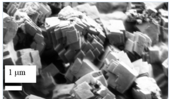
Figure 12. SEM images of whitlockite crystallites.
