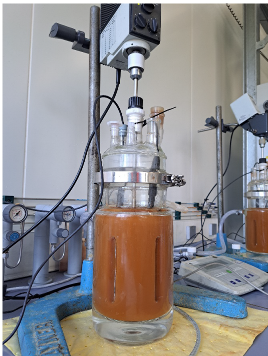
Figure 2. Photograph of the experimental setup using 2 L reactors.
