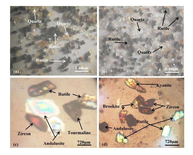
Figure 2. Morphological aspects of some heavy minerals (rutile, quartz, tourmaline, and alusite, zircon, brookite and kyanite): hand samples (a-b) and under the binocular magnifying glass (c-d).
