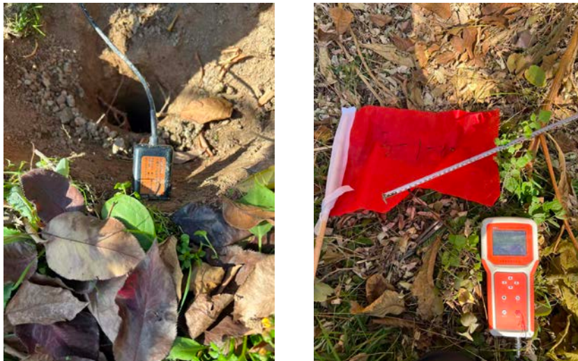
Fig. S5 Photos of the sensor (left) and instrument (right) used for measuring soil parameters (SN-3001-TRREC-N01, Shandong Renke Control Technology Co., Ltd.).
