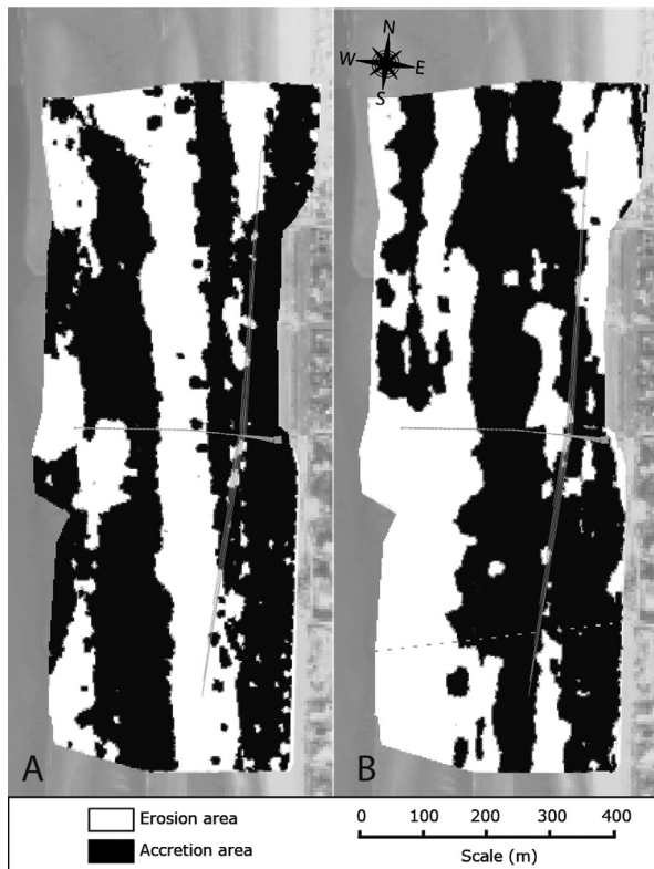
Fig. 10. Example of cut and fill maps. A. Period before drainage system installation (June 2008–December 2008). B. September 2012–September 2013.
