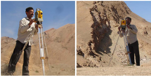
Fig. 5. In situ field measurement using the Total Station surveying equipment (Trimble™5600).
