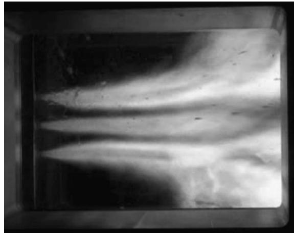
Cryogenic flames formed by three coaxial injectors fed with liquid oxygen and gaseous methane. Combustion is coupled with acoustic perturbations at the first transverse mode of the chamber. (Photo: F. Richecoeur, P. Scouflaire, S. Ducruix and S. Candel, EM2C, CNRS and L. Vingot, Onera)
