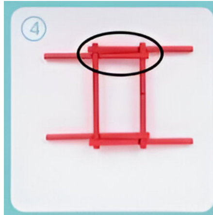
Figure 2. Reciprocal unit circled in black on the simplest form of the Da Vinci bridge.
