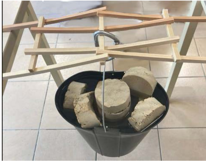
Figure 12. Image of the test setup in the case of a bridge composed by square cross-section wooden beams.
