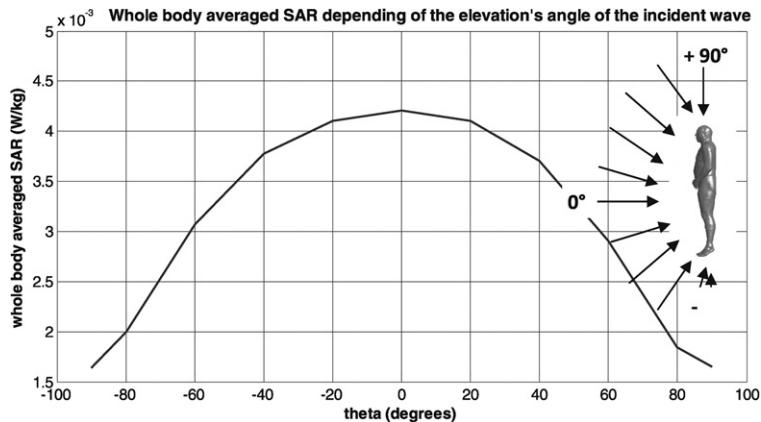
Whole body SAR induced in VH at 2100 MHz for V-polarization depending on the angle of arrival in a vertical font plane (see Conil et al. this issue).
