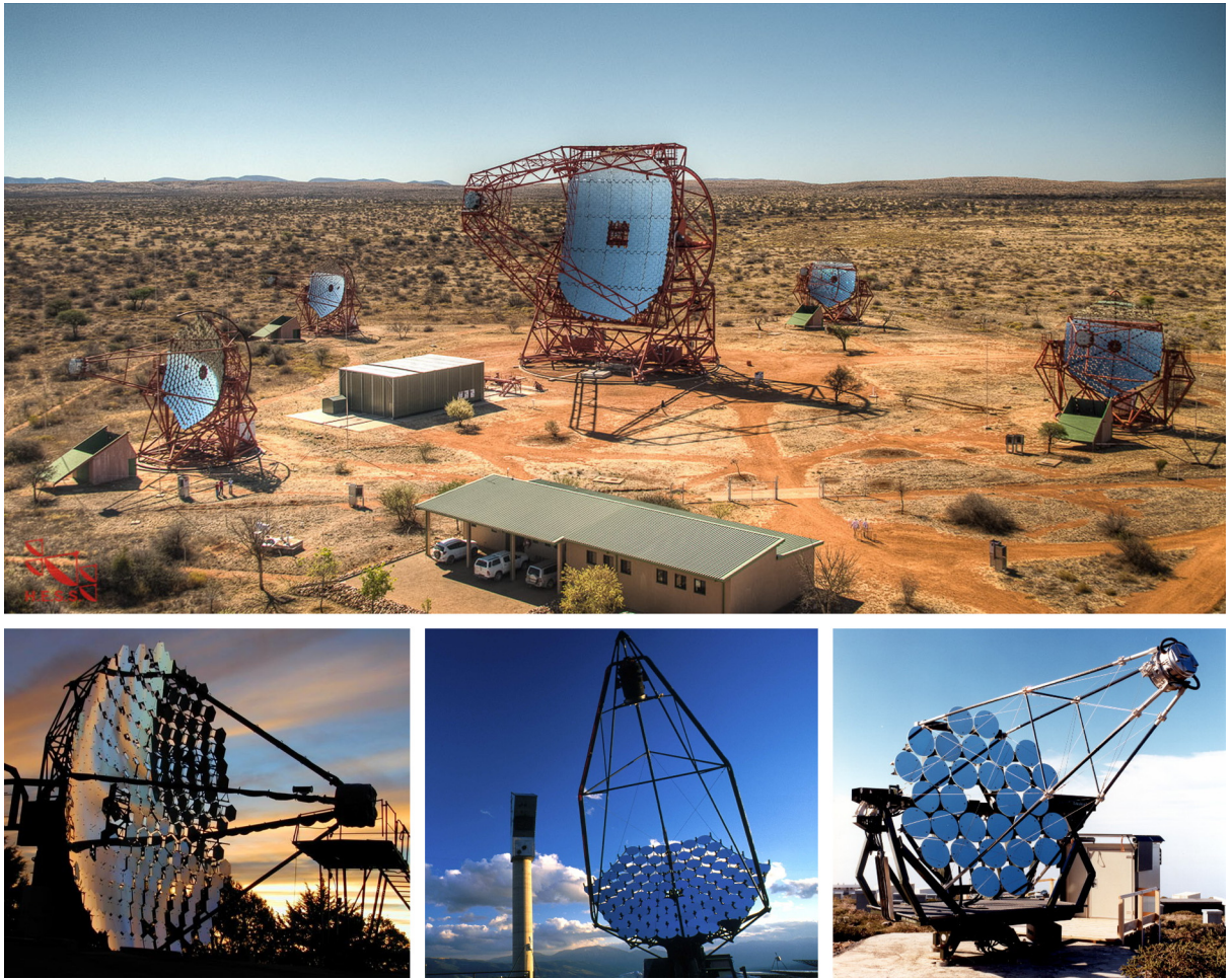
Fig. 5. (Color online.) Illustration of the combination in H.E.S.S. (upper panel) of large dishes as in Whipple (lower left), fast and fine grained cameras as in CAT (lower center) and stereoscopic observation as in HEGRA (lower right)]. Image credits: Christian Föhr, MPIK for the H.E.S.S. array; Steve Fegan for the Whipple telescope; Olivier Blaise for the CAT telescope; German Hermann, MPIK for the HEGRA experiment.
