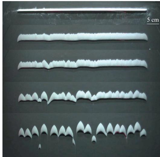
**Figure 6.** Instability of an isolated transverse ridge migrating on a starved bed. Flow is from top to bottom (translated tray setup). Images were taken after none, 40, 100, 200, 400, and 800 tray strokes. Images are from [86].
