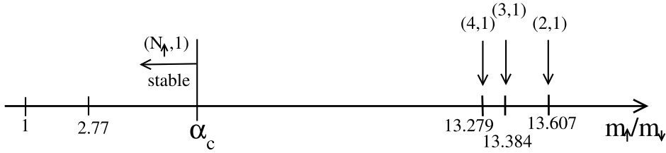
Figure 3. Known results on the stability of the (N_\uparrow, 1) system of N_\uparrow spin \uparrow fermions and one spin \downarrow fermion, for a zero-range interaction, as a function of the m_\uparrow/m_\downarrow mass ratio between a \uparrow particle and the \downarrow particle. Vertical arrows: critical values of m_\uparrow/m_\downarrow (thresholds) for the (N_\uparrow, 1) -body Efimov effect obtained by solving the corresponding problem, see references [39] for N_\uparrow = 2 , [30] for N_\uparrow = 3 , [40] for N_\uparrow = 4 ; when m_\uparrow/m_\downarrow exceeds these values, the energy of the system is no longer bounded below. Vertical bar with horizontal arrow: critical mass ratio \alpha_c , whose existence is established by the Moser–Seiringer theorem [41], below which the system (N_\uparrow, 1) is stable \forall N_\uparrow ; the theorem does not give the exact value of \alpha_c but a more restrictive lower bound, \alpha_c > 2.77 , than that, m_\uparrow/m_\downarrow = 1 , of the cold-atom experiments (a superiority of the latter, however, is that the unitary Fermi gas appears to be stable, without collapse or significant three-body losses, for all values of N_\uparrow and N_\downarrow ).
