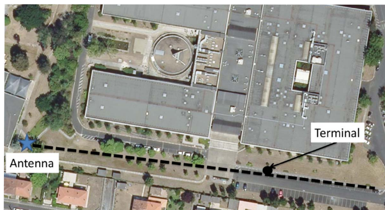
Figure 1. Satellite view of the Mérignac measurement site with the positioning of the antenna, the UE which receive the data sent by the antenna and the measurement axis in black.
