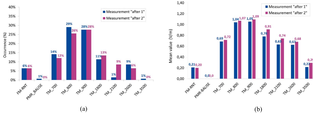
Figure 5. Distribution of main contributions to overall exposure (a) by service/frequency band and evolution of their mean value (b). (FM-RNT: Radio broadcasting, PMR-Balise: Private Mobile Radio, TM: Mobile Telephony (cellular network).)
